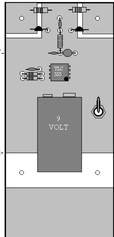
Fig. 3 - PCB component layout.
