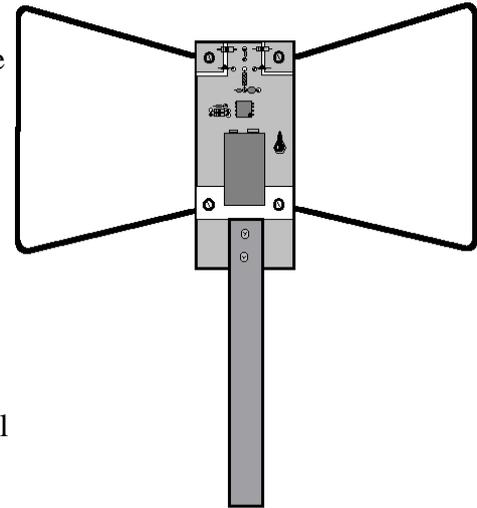
Fig. 1 - The assembled TDOA antenna unit - coaxial cable to receiver runs behind the PCB and through the PVC pipe handle.
